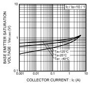
Fig.7 Base-Emitter Saturation Voltage vs. Collecter Current
