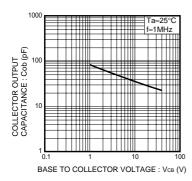
Fig.10 Collector Output Capacitance
